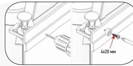
**[EN] ATTENTION!** The steps listed below show the basic installation of the product. The order of the steps may differ depending on the utility systems and the size of the premises. Step 1 to perform when you buy tray disassembled form.
